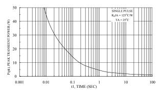
Figure 10. Single Pulse Maximum Power Dissipation
