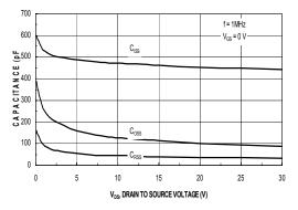
Figure 4. Capacitance Characteristics
