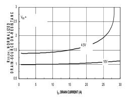
Figure 3. On Resistance Vs Vgs Voltage
